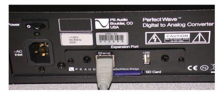
Check to see if the Bridge requires a firmware update. To do this you must be connected to the Internet. Once connected, go to the Input Select screen on the PWD's touch screen. On the Media Bridge input select choice, touch the green edit icon on the right hand side. This brings you to the Bridge setup page where you can touch the option to upgrade the firmware. Once upgrading DO NOT REMOVE POWER WHILE THE BRIDGE IS UPDATING.
