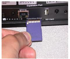
Note: This SD card plugs into the socket with the gold contacts facing up. Make sure the SD card has the gold contacts facing up, or the socket could be damaged.
