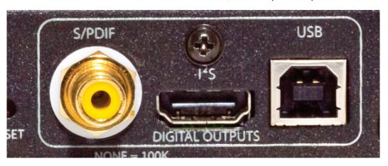
I<sup>2</sup>S contains separate clocks and data lines and does not have jitter related issues. Most jitter problems arise from the use of the S/PDIF protocol because compressing the native I<sup>2</sup>S data and clocks together into one stream and then unravelling this compressed format back to I<sup>2</sup>S (as is required for it to work) is typically where jitter is introduced. I<sup>2</sup>S should be the transmission medium of choice if you have a compatible receiver to accept it.
