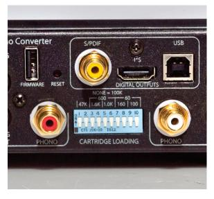
pull the unit out again. The system is easy to select. With all the switches down, the cartridge loading is quite high at 100K Ohms. To set the load, simply push the appropriate switches to the up position. The switches must be moved in pairs (one for the left and one for the right channel). For Moving Magnet cartridges, the typical load will be 47K. Move switches 1 and 2 up, keeping
