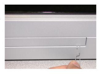
object near the right side, beneath the disk tray as shown, and push inwards until the drawer mechanically releases. This will allow you to pull the drawer open the rest of the way and remove the disc. Return power to the PWT and press the touch screen eject/insert icon to return to normal operation.
